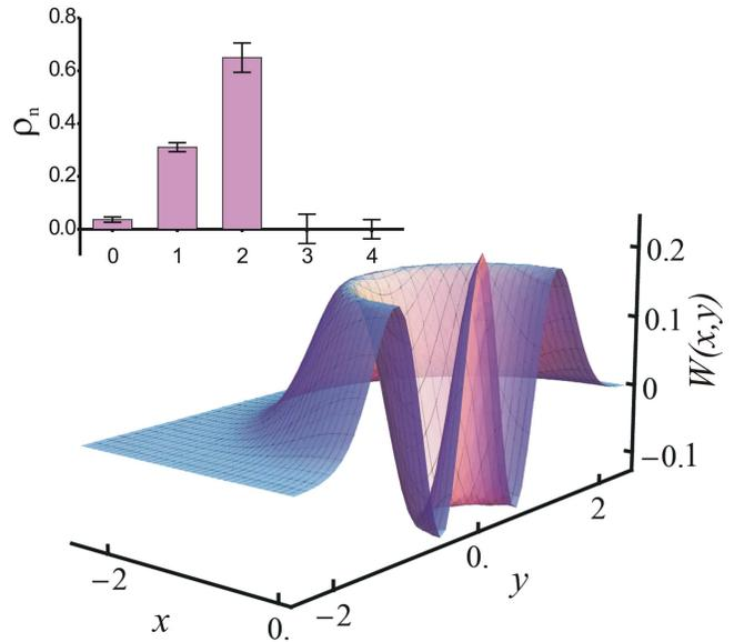
FIG. 2: (color online) Experimentally reconstructed density matrix diagonal elements and corresponding Wigner function for the two-photon Fock state generated by cavity-enhanced SPDC.
