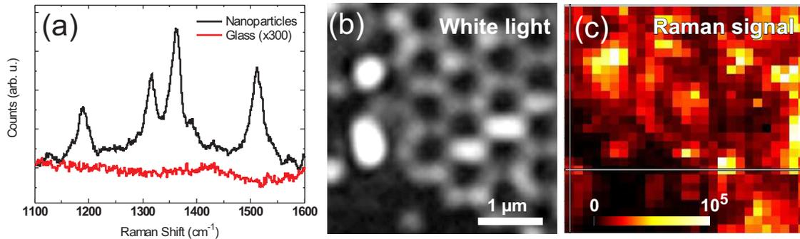
Figure 5. (a) Raman spectra from R6G on nanoparticles and glass. (b) Reflected white light image of nanoparticle array. (c) Intensity map of the  $1500\text{ cm}^{-1}$  Raman line, from a region similar to (b).
