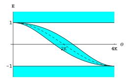
FIG. 1: Band spectrum of the BdG Hamiltonian (4) for the complex crystal condensate (13), as a function of the twist parameter  $\theta$ . The dashed line denotes the infinite period limit [in this case  $\nu \to 0$ ], which is Shei's solution (11). At  $\theta = 2\mathbf{K}$  we recover the symmetric spectrum of the real kink crystal, relevant to the GN<sub>2</sub> system.
