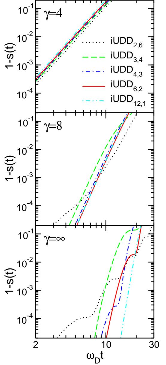
FIG. 3: Comparison of the performance of various iterated  $i\text{UDD}_{m,c}(t)$  sequences for a total number of  $n = 12$  pulses and various cutoff exponents  $\gamma$ . Other values are  $\alpha = 1/4, T = 0$ .
