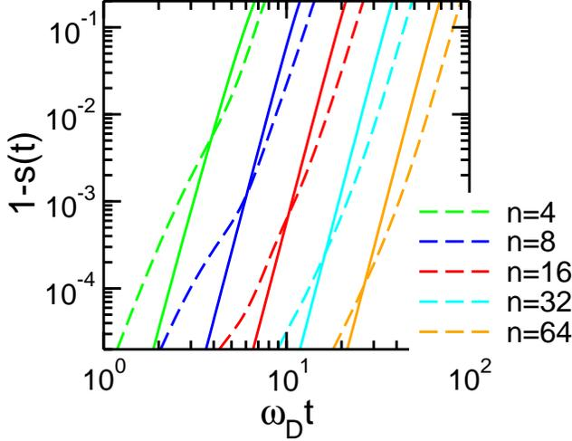
FIG. 2: Comparison of the performance of the CPMG (dashed lines) and the UDD sequence (solid lines) for various number of pulses  $n$  (legend holds for dashed and solid lines) and a spectral density with  $\gamma = 8$  corresponding to a cutoff of intermediate hardness. Other values are fixed:  $\alpha = 1/4, T = 0$
