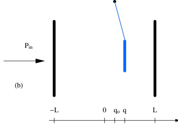
FIG. 1: The three-mirror cavity arrangement. The two outer mirrors are fixed and the middle mirror vibrates harmonically about its equilibrium position  $q_0$ .  $P_{in}$  is the laser power coupling into the cavity.
