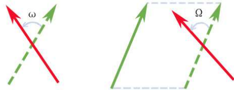
FIG. 1: (Color on line) The left scheme depicts the time evolution of \vec{N} at a point \mathbf{r} ; the right scheme illustrates the spatial deviation of \vec{N} by comparing the fields at two neighborhood points \mathbf{r} and \mathbf{r} + \Delta\mathbf{r} for which the parallel displacement is inevitable.
