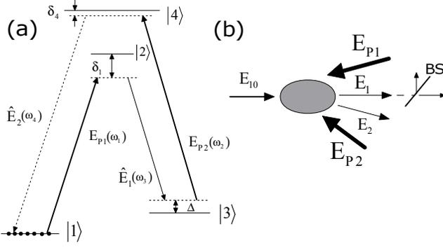
FIG. 1: (Color online) (a) Schematic atomic level diagram.  $E_{P1}(\omega_1)$  and  $E_{P2}(\omega_2)$  are the pump fields, and  $\hat{E}_1(\omega_3)$  is the probe field.  $\hat{E}_2(\omega_4)$  describes the process of another photon ( $\omega_4$ ) generated by FWM. (b) Schematic of the experiment for 2+1 photons generation.
