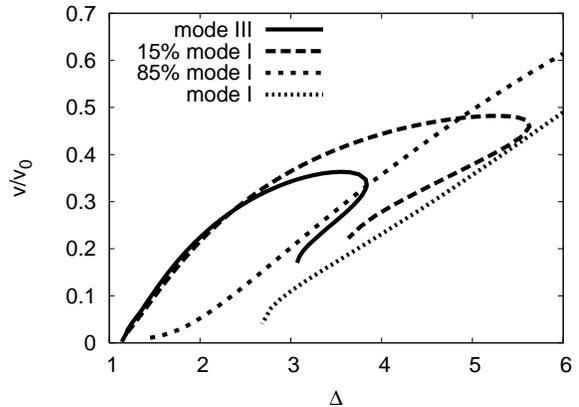
FIG. 2: Steady state propagation velocity as function of the driving force for pure mode III and mode I fracture. Additionally, mixed mode situations with  $\Delta_I/\Delta = 0.15$  and  $\Delta_I/\Delta = 0.85$  are displayed. The velocity scale is  $v_0 = (D\tau_0^{-3})^{1/4}$ .
