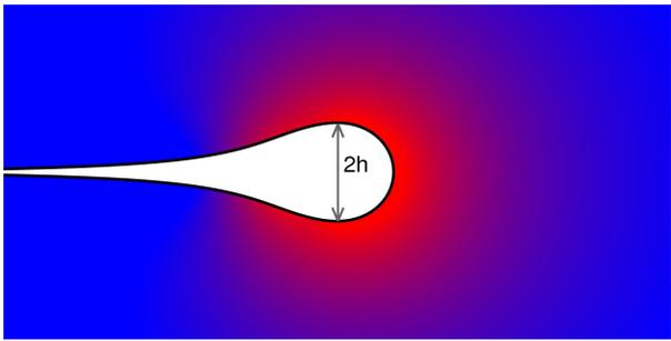
FIG. 1: Shape of a mode III crack for  $\Delta = 2.5$  in the steady state regime. The total incoming elastic energy flux is converted into surface energy, surface dissipation and viscous bulk dissipation, which is localized to the scale  $v\tau_0$  around the crack tip (visualized by the color coding).
