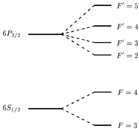
FIG. 2: Level diagram for Cesium. The two hyperfine ground state manifolds  $6S_{1/2}, F = 3$  and  $6S_{1/2}, F = 4$  correspond to manifolds  $a$  and  $b$  in our theory, and one of the excited state hyperfine manifolds, either  $6P_{3/2}, F' = 3$  or  $6P_{3/2}, F' = 4$ , corresponds to manifold  $e$ .
