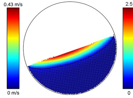
FIG. 1: Time averaged velocity field in the simulated 2D rotating drum. In this peculiar numerical experiment, the rotation speed was  $\Omega = 6$  rpm. The black line shows the interface between the flowing layer and the “static” packing. Velocities are expressed in  $m/s$  (left-hand colorbar) or non-dimensionalized by  $\sqrt{gd}$  (right-hand colorbar) where  $g$  refers to the gravity constant and  $d$  to the mean diameter of the beads (see text for details).
