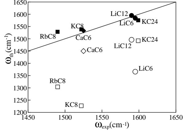
FIG. 1: Calculated adiabatic (empty symbols) and non-adiabatic (filled symbols)  $E_{2g}$  phonon frequencies of several GICs, compared to the available experimental data. The full line represents the experimental values.
