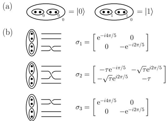
FIG. 1: (a) Basis states for the two-dimensional Hilbert space (a qubit) spanned by two pairs of anyons with total topological charge 0, where the black dots denote the nontrivial anyons in the Fibonacci model. (b) Braiding matrices for the qubit, where  $\tau = (\sqrt{5} - 1)/2$ . The anyons are labeled 1 to 4 from left to right in (a) and from bottom to top in (b).
