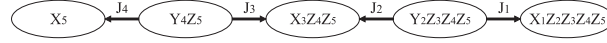
Fig. 2. Oriented graph summarizing the recurrence formulas to obtain the operator decomposition for a 5-qubit chain, whose Hamiltonian reads \hat{\mathcal{H}} = \sum_{i=1}^4 J_i(\hat{X}_i\hat{X}_{i+1} + \hat{Y}_i\hat{Y}_{i+1}) .
