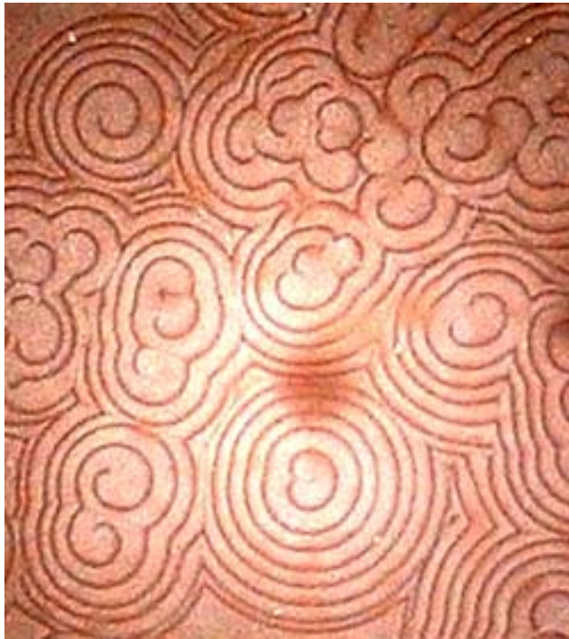
Figure 3: Enlarged photo of spiral wave-fronts in precipitating systems: copper chloride and potassium hydroxide. Size is 1 \times 1mm [4].
