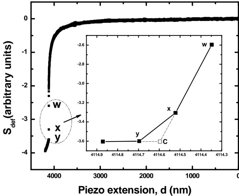
Figure 5: The measured  $S_{def}$  corresponding to the electrostatic force due to an applied voltage between the sphere and plate as a function of the distance moved by the plate  $d$  is shown as squares. The region around the sphere-plate contact is shown in the inset. The slope of the line  $WX$  from the two data points preceding contact can be extrapolated to obtain an accurate value of the contact position  $C$  as explained in the text.
