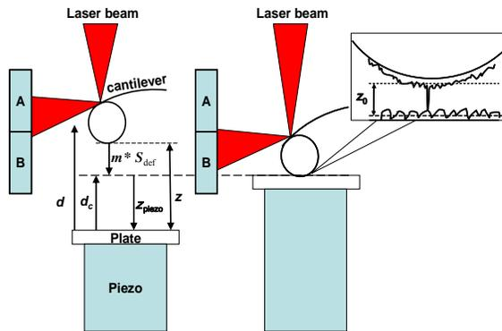
Figure 1: Schematic of setup used. The extension of the piezo is given by  $d$ , with  $d_c$  being its value at the point of sphere-plate contact,  $z_{piezo}$  is the distance moved by the plate measured from contact,  $z_0$  is the average separation on contact,  $m$  is the deflection coefficient and  $S_{def}$  is the deflection signal.
