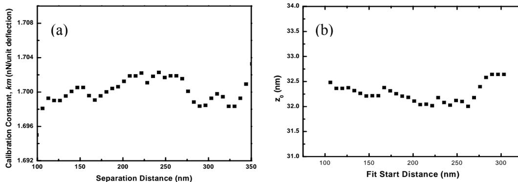
Figure 7: (a) The cantilever calibration constant  $k'$ , and (b) the average separation on sphere-plate contact  $z_0$ , obtained from fitting the  $X(z)$  as a function of the start point of the fit. Note the random variation of the values with the separation distance, which is indicative of the absence of systematic errors in the fit.
