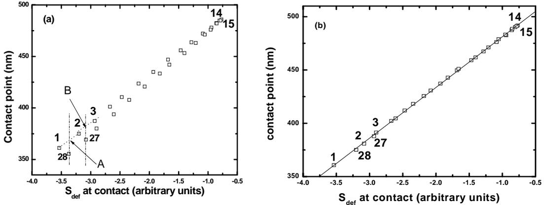
Figure 6: (a) The contact point  $d_c$  and deflection signal  $S_{def}$  at sphere-plate contact of the electrostatic force curves such as in figure 5. The numbers indicate the time sequence corresponding to the electrostatic force curves obtained by applying dc voltages to the plates. In (b) the contact points have been corrected for thermal and mechanical drift in the system.
