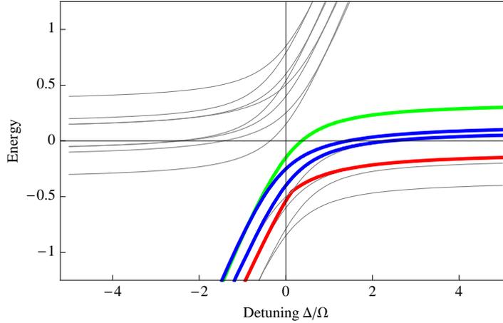
**Figure 4.** Example of eigenspectrum as a function of the detuning  $\Delta$  for typical parameters. The eigenstates tending to the computational basis states for  $\Omega/\Delta \rightarrow 0$  (i. e. to the far right in this figure) are colour-coded as follows:  $|00\rangle$ : green,  $|10\rangle$  and  $|01\rangle$ : blue,  $|11\rangle$ : red.
