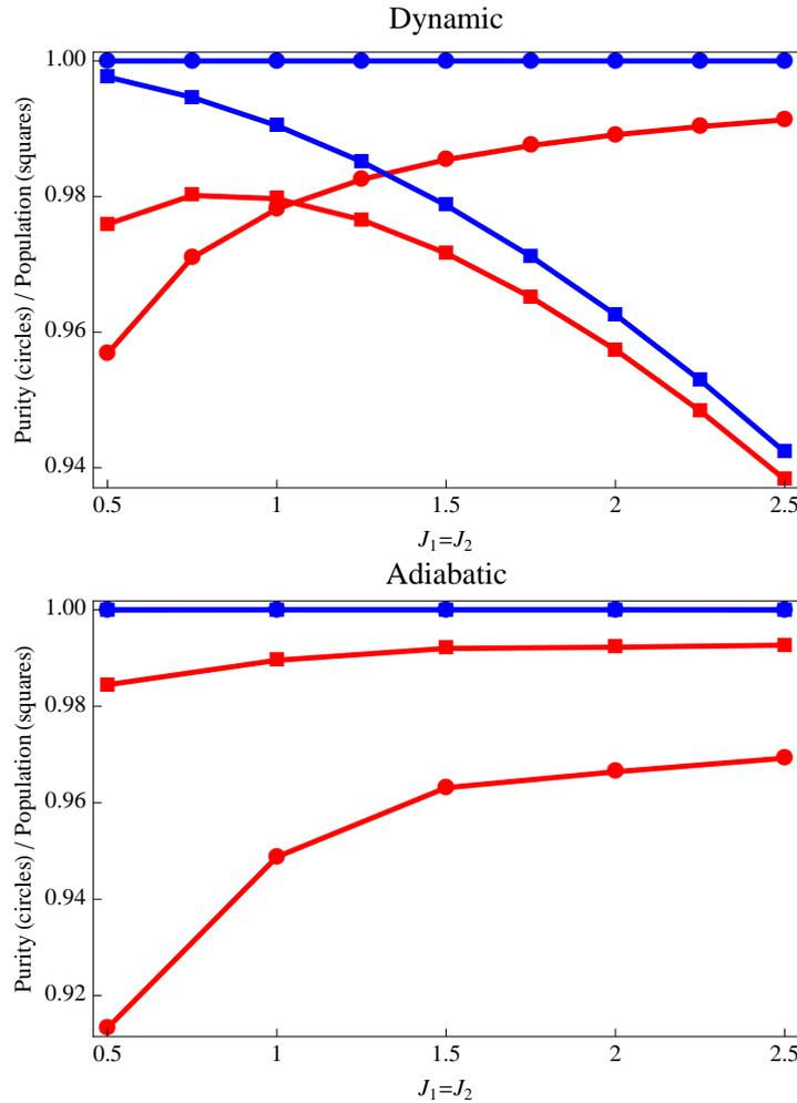
**Figure 9.** Intrinsic gate errors (blue curves) and additional effects of decoherence (red curves): the final purity and the final population of the computational basis states are shown as a function of the coupling strength  $J_1 = J_2$  (in units of  $0.1 \text{ ps}^{-1}$ ). A decay rate of  $1 \text{ ns}^{-1}$ ,  $R = 1.2$  and typical laser pulse parameters have been used.
