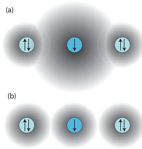
**Figure 1.** In the optical ground state of the central control qubit (b), the wavefunctions of the three species do not overlap and there is no spin-spin exchange interaction. When the central control is optically excited (a) its wavefunction has a larger extent and so activates the spin-spin coupling.
