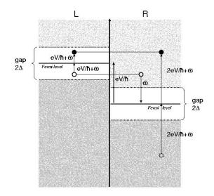
FIG. 12: Illustration of Andreev reflection as mirroring at the Fermi levels for electron-hole conversion and vice versa. For either side the incoming and reflected levels can lie inside or outside the gap. Only the beginning and end of a complete multiple-reflection process have to be in the electron or hole reservoir below or above the gap, respectively.
