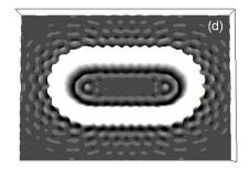
FIG. 3: (a) Top view of the structure: gold pads (90x90x30nm) on a glass subtrate. Calculated densities of states  $\rho_{xx}$  (b)  $\rho_{yy}$  (c) and  $\rho_{zz}$  (d) in a plane 100nm above the substrate for wavelength  $\lambda = 543$ nm [reproduced after [19]]. The grey scale is from -50 to 35 in (b), -45 to 30 in (c), -7.5 to 15 in (d) and higher or lower values are white or black, respectively.
