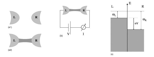
FIG. 4: A left and a right bulk reservoir, uncoupled (a1) and coupled (a2). (b) Contact as embedded in a circuit. (c) Fermi levels left and right with applied voltage. The dotted line marks a fixed energy over both sides.
