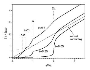
FIG. 13: Calculated current-voltage curves for transport channels of three different transmissions (normalized to  $\theta$ ) [reproduced after [58]]. The normal conducting IV is added for comparison (keep  $\Delta$  just for units).
