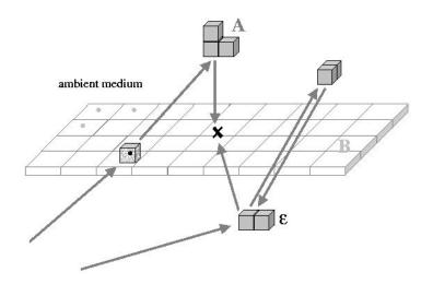
FIG. 1: Objects distributed in space and discretized into cubes of equal size. A plane in space discretized into a quadratic mesh is also shown. Arrows indicate only some possible scattering paths to a location marked by the cross.
