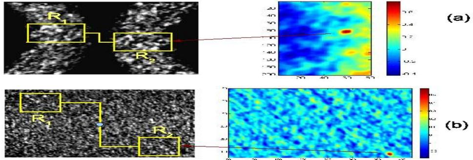
Fig. 2. Spatial correlation between signal and idler down converted light with interference filter around degeneracy(a) and without a narrow filter (b). In each row the first inset is a ccd image, the second a plot of the cross correlation function. The axis report the pixels position in the CCD array.  $C_{12}(\xi)$ .
