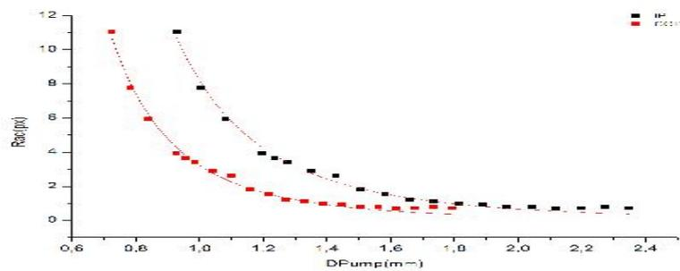
Fig. 4. Observed dependence of the radius (in pixels) of the speckles from the pump diameter. The two curves differs in the estimation of the pump diameter: in one case it was measured with an impact paper (IP) and in the other case with a CCD.
