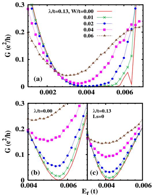
FIG. 3: (Color online) Conductance vs Fermi energy with different disorder strengths  $W$  in the vicinity of the antiresonance energy gap. (a) with both the Fano antiresonance and the structure antiresonance; (b) with only the structure antiresonance; (c) with only the Fano antiresonance.
