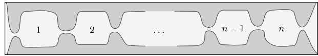
FIG. 1: (Color online) Schematic drawing of an array of n chaotic cavities. The cavities are connected via ballistic contacts with dimensionless conductance g_c . The semiclassical theory requires the limit g_c \rightarrow \infty at a fixed ratio n/g_c .
