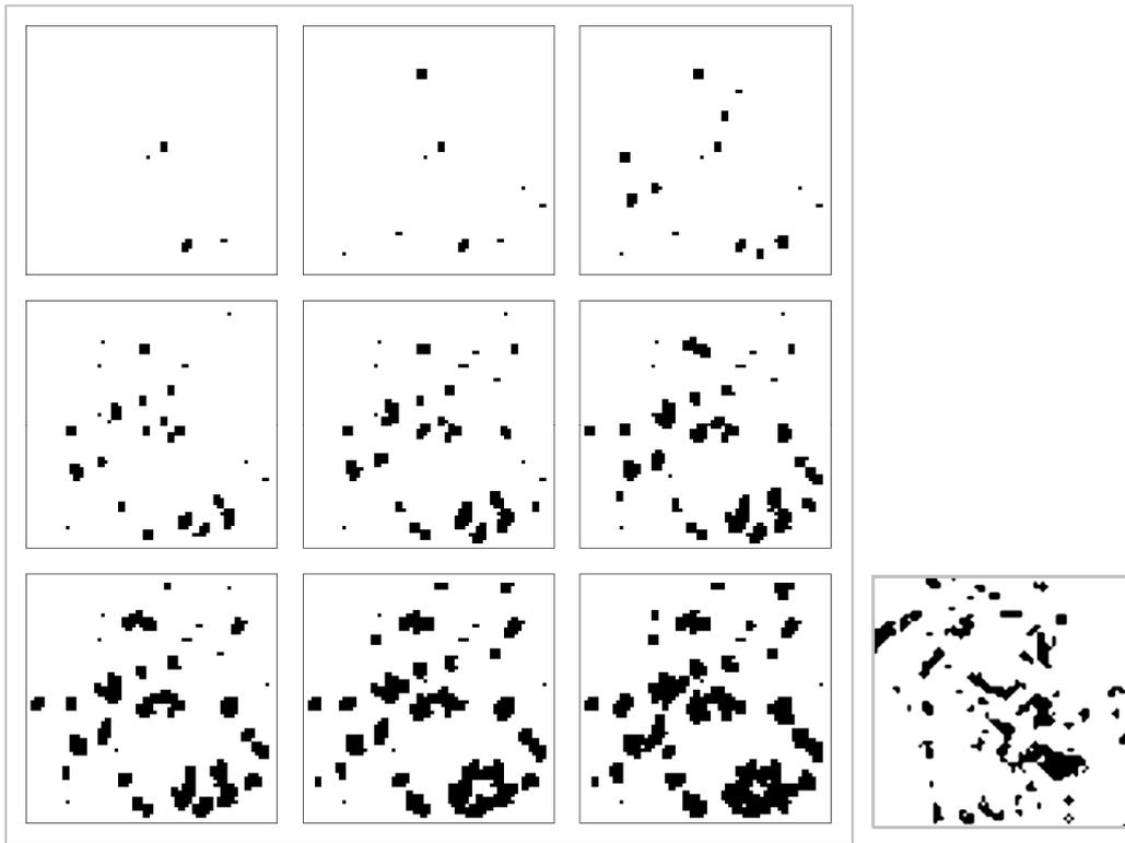
Figure 7: Construction of the 2-D binary image of pore architecture (left panel) based on complex network model with preferential attachment rule for pore connectivity. Left panel shows the progressive build-up of the image as new pores are introduced to the image. The simulation is stopped when the desired porosity is achieved. Image on the right is the actual 2-D X-ray CT scan of the soil sample.
