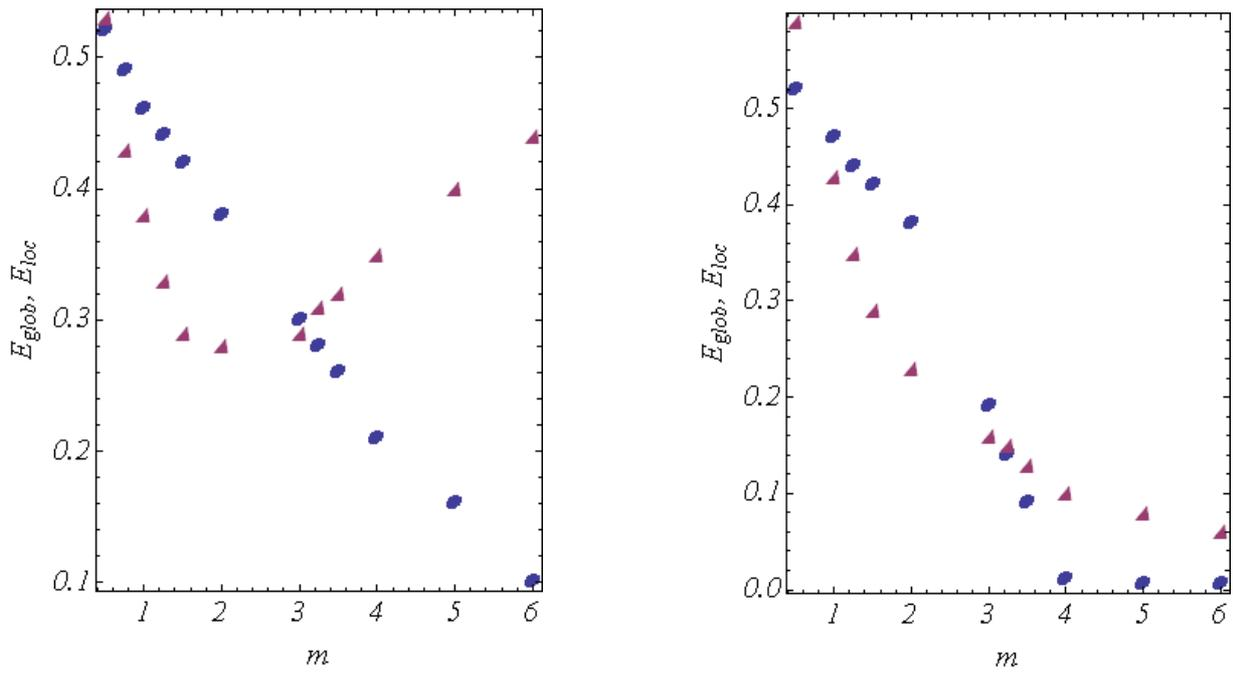
Figure 4: Dependence of local (triangles) and global (dots) efficiency of the pore network on the value of the exponent in the definition of connectivity (eq. (2)). Left: networks constructed with constant number of edges (=2000). Right: networks constructed with constant number of vertices (=400).
