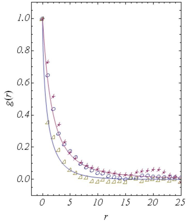
Figure 8: Normalized two-point correlation function for the simulated soil image (stars), the actual X-ray CT scan (open dots) and for the random image with the same porosity. The full lines are the plots of the correlation functions according to eq. (9) and (10) with  $r_0 = 4$ ,  $s=2,3$  for the soil and for the simulated soil image, and  $r_0=1$ ,  $s=0,65$  for the random image.
