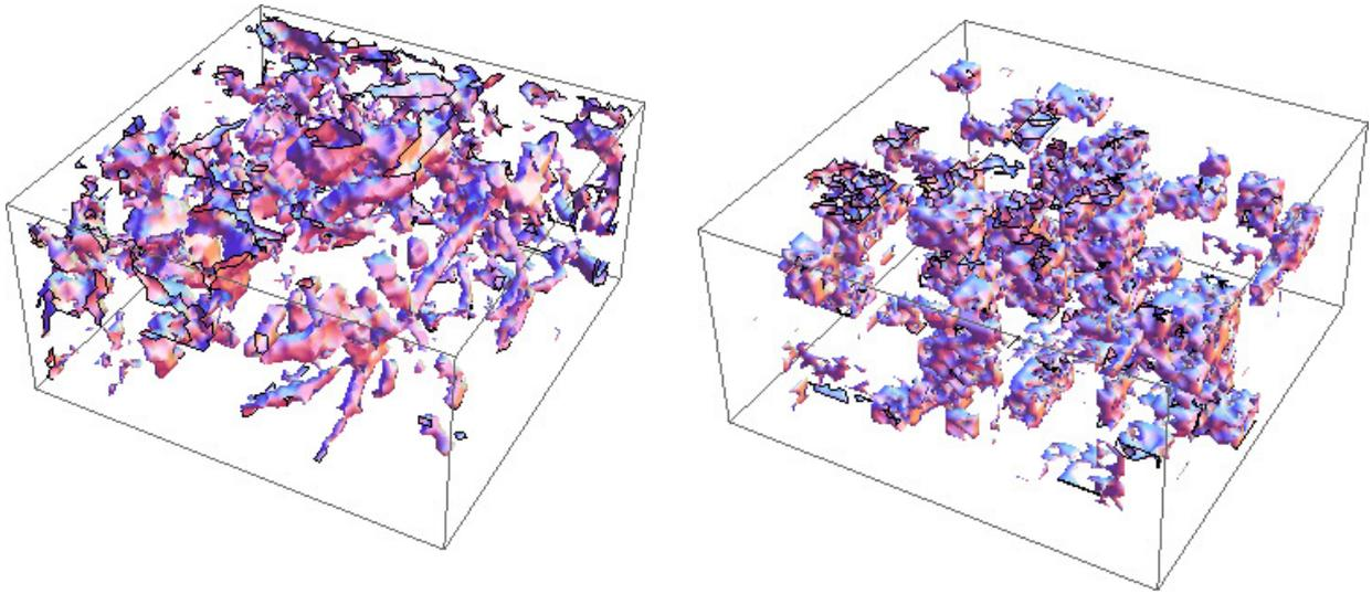
Figure 9: Left: 3-D reconstruction of the soil pore architecture from stack of X-ray CT scans. The pore space is shown while the soil matrix is here transparent. Right: 3-D model of the soil pore architecture based on the pore complex network with preferential attachment rule for the pore connectivity.
