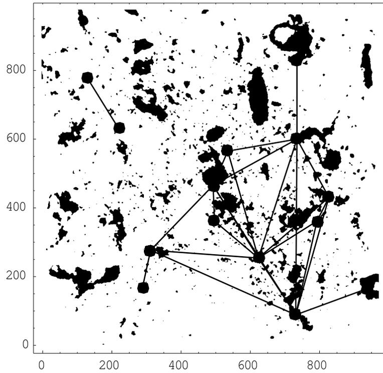
Figure 1: 2D X-CT binary image of undisturbed soil sample. Pores are shown as black areas. Superimposed on the soil image is the constructed network at high cut-off value (i.e. small number of edges) for the pore connectivity (eq. (2)) with  $m=1$ .
