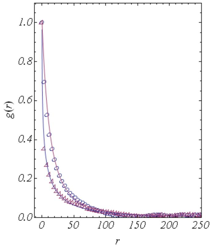
Figure 6: Two-point normalized correlation function of the soil pore structure computed from the soil image in fig.1 (open dots) and for the random image with the same porosity. The solid lines are plots of eqs. (9) and (10) with  $r_0 = 27$ ,  $s = 2,2$  for the soil image, and  $r_0 = 4$ ,  $s = 0,4$  for the random image.
