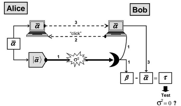
FIG. 3: **Control mode (CM)**. Alice picks up a Gaussian amplitude  $\bar{\alpha}$  and prepares a signal coherent state  $|\bar{\alpha}\rangle$ . Such a state is sent to Bob, who heterodynes it with outcome  $\beta$  (step 1 in the picture). Then, Bob classically informs Alice (step 2) and Alice communicates the value of the signal  $\bar{\alpha}$  (step 3). At that point, Bob computes the test variable  $\tau := \beta - \bar{\alpha}$  and tests the noise of the channel.
