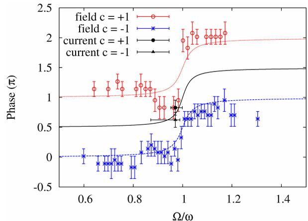
FIG. 3: (color online) Phase response of magnetic vortex oscillators as detected by time-resolved X-ray microscopy normalized to the respective resonance frequency. The red circles and the blue stars represent the phase responses of two permalloy squares excited purely by an AC-magnetic field. The black circle and triangle represent the phases of the current-fluxed samples shown in Fig. 2(b) and (c), respectively.
