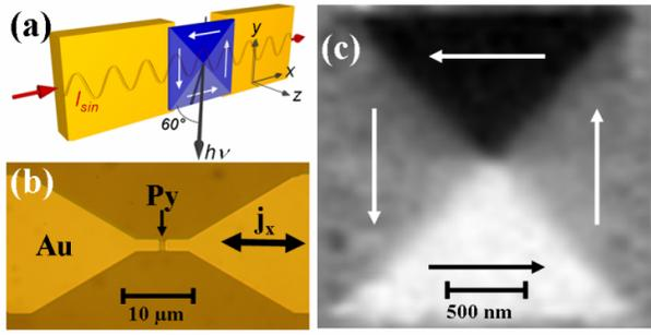
FIG. 1: (color online) (a) Scheme of the permalloy square contacted by two gold wires. The sample is tilted by  $60^\circ$  relative to the incident X-ray beam. (b) Optical micrograph of a permalloy square and its contacts on the  $\text{Si}_3\text{N}_4$ -membrane. (c) Magnetic contrast of the relaxed permalloy square with a thickness of 20 nm showing the  $x$ -component of the magnetization as black-to-white contrast.
