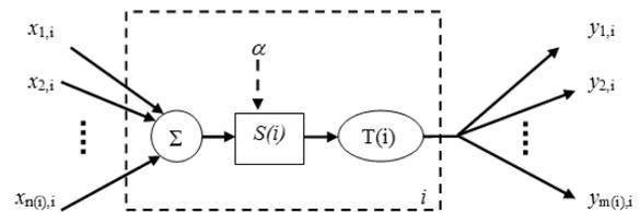
FIG. 1: The integrate-and-fire neuronal cell adopted in the previous works [32, 33] incorporates three stages: (i) integrating of input activations; (ii) memory of activation  $S(i)$ ; and (iii) non-linear transfer function involving a threshold  $T(i)$  (a hard limiter). While those previous works adopted full conservation of the activation (i.e. decay rate  $\alpha = 0$ ), in the present work the stored activation undergoes exponential time decay with rate  $\alpha$ .
