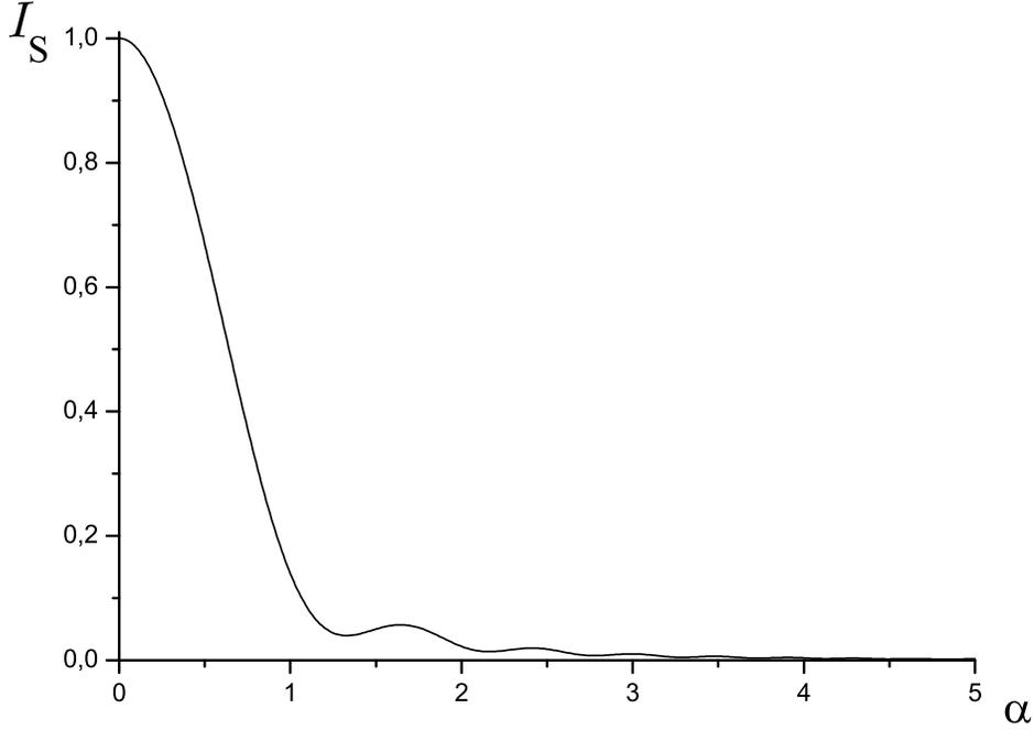
Fig. 12. The universal function  $I_S$ , used to calculate intensity at the virtual-source position.
