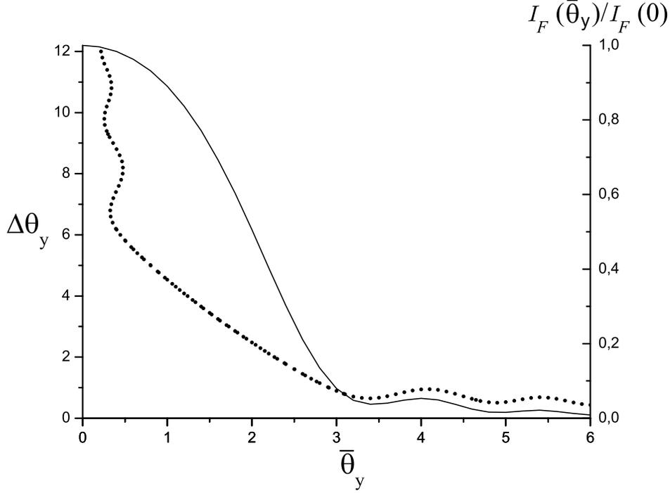
Fig. 16. Comparison between some zeros of  $\mathcal{X}_F$ , at coordinates  $(\bar{\theta}_y, \Delta\theta_y)$  (black circles), and the directivity diagram of undulator radiation in the vertical direction at very large horizontal electron beam divergence  $\hat{D}_x \gg 1$  and negligible vertical divergence  $\hat{D}_y \ll 1$  (solid line).
