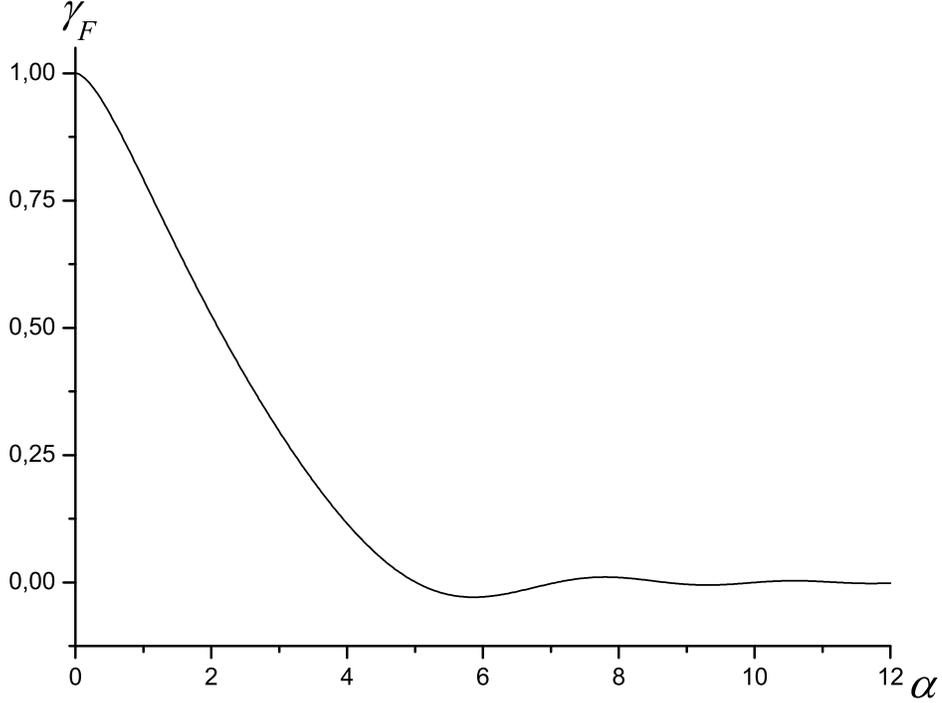
Fig. 20. Plot of the universal function  $\gamma_F$ , used to calculate the cross-spectral density in the far zone when  $\hat{N}_x \gg 1$ ,  $\hat{D}_x \gg 1$ ,  $\hat{N}_y \lesssim 1$  and  $\hat{D}_y \gg 1$ .
