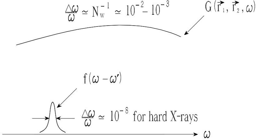
Fig. 3. Schematic illustration of the relative frequency dependence of the spectral correlation function  $\bar{f}(\omega - \omega')$  and of the cross-spectral density function (the cross-power spectrum)  $G(z, \vec{r}_1, \vec{r}_2, \omega)$  of SR at points  $\vec{r}_1$  and  $\vec{r}_2$  at frequency  $\omega$ .
