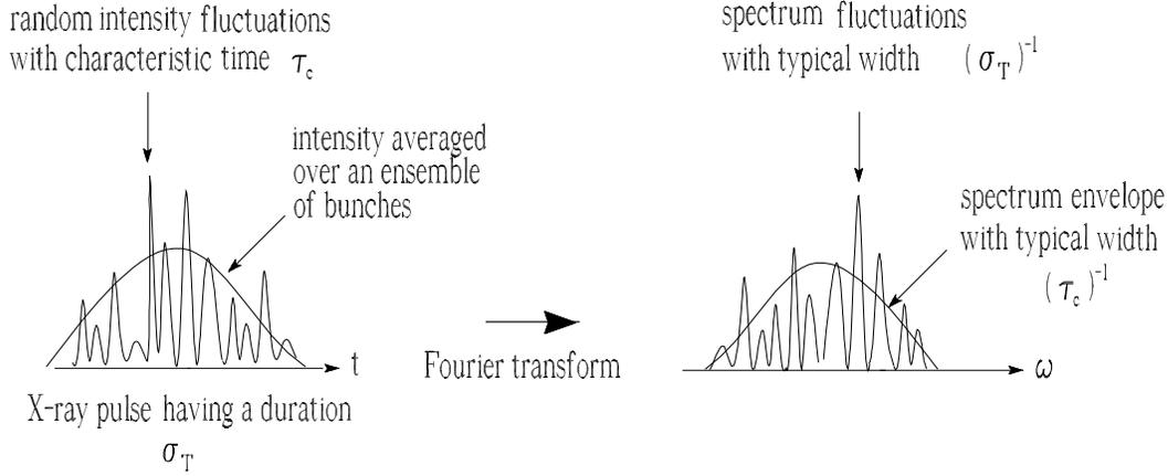
Fig. 5. Reciprocal width relations of Fourier transform pairs.
