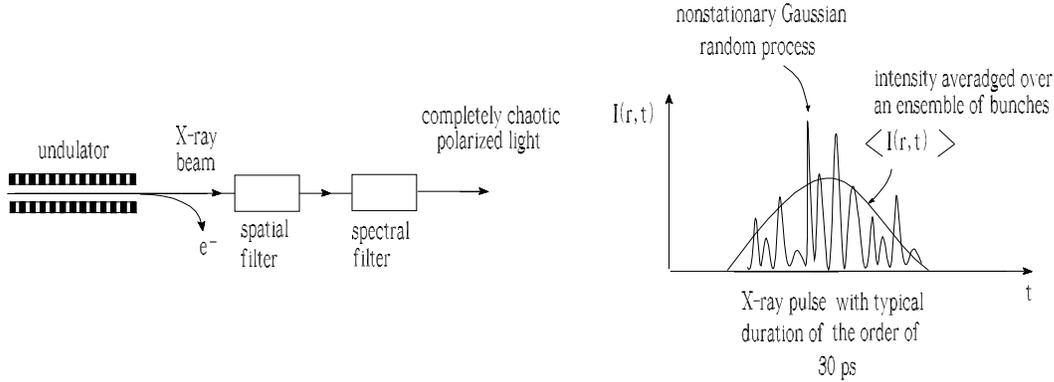
Fig. 2. The intensity of an X-ray beam from a SR source. A statistically non-stationary wave has a time-varying intensity averaged over an ensemble of bunches.
