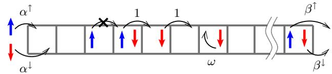
**Fig. 1.** (Color online) Illustration of an exclusion model with two internal states, denoted as spin-up ( $\uparrow$ ) and spin-down ( $\downarrow$ ). Particles are injected at the left boundary at rates  $\alpha^\uparrow, \alpha^\downarrow$ , and extracted at the right at rates  $\beta^\uparrow, \beta^\downarrow$ . Within bulk, particles move unidirectionally to the right, or flip their state (at rate  $\omega$ ), always obeying Pauli's exclusion principle.
