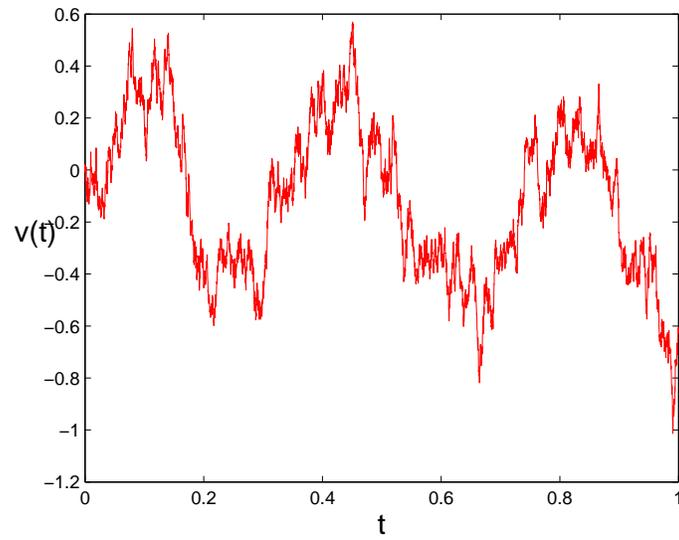
Figure 3: Velocity Plots at length scales where viscosity is dominant
