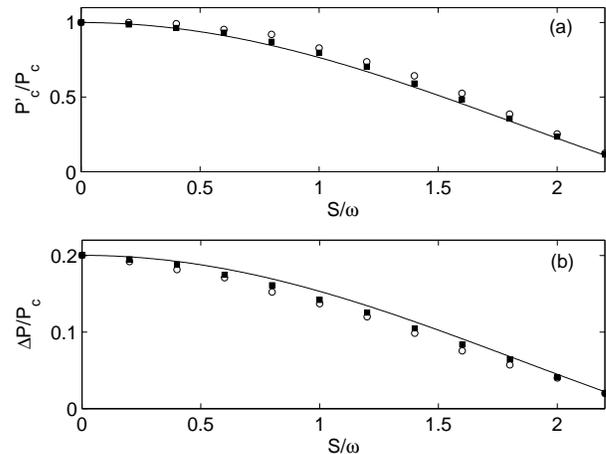
FIG. 3: (a) Threshold switching power as a function of the ratio  $S/\omega$ . (b) Switching width as a function of the ratio  $S/\omega$ . The open circles are for  $\omega/v = 10$ , the squares are for  $\omega/v = 20$ , and the solid lines represent the theoretical results at the high frequency limit.
