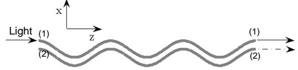
FIG. 1: Schematic drawing of a periodically curved all-optical switch. The two curves represent two waveguides. The laser light switches its output waveguide when the laser power is changed from above to below a threshold value.
