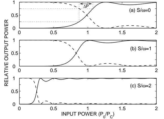
FIG. 2: Relative output powers as functions of the input power for three different values of  $S/\omega$  at  $\omega/v = 10$ . The solid lines are for the launching waveguide while the dashed lines are for the neighboring waveguide. The input power  $P_0$  is scaled by the threshold switching power  $P_c$ .
