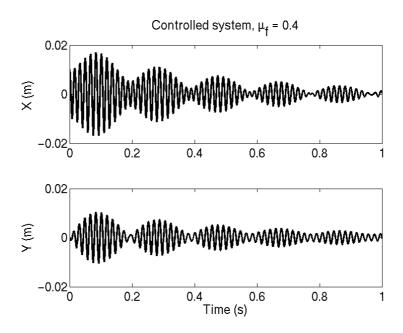
Figure 18 : Temporal response of the controlled system for  $\mu_{\scriptscriptstyle f}$  = 0.4
