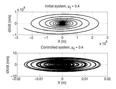
Figure 19 : Divergent oscillations for  $\mu_f = 0.4 \, \left( \mu_{f0} < \mu_f < \tilde{\mu}_{f0} \right)$
