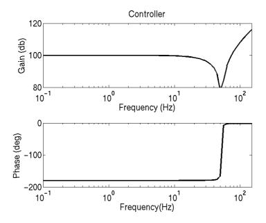
Figure 5 : Bode diagram of the controller
