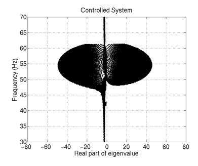
Figure 16 : Frequency and real part of eigenvalue of the controlled system for various friction coefficient  $\mu_f$  and stiffness  $k_1$
