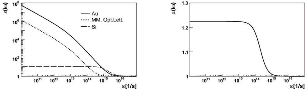
FIG. 3: Left panel:  $\varepsilon(i\omega)$  for meta-material discussed in [16] in comparison with gold and silicium. Right panel: the magnetic permeability of the meta-material  $\mu(i\omega)$ ;  $\mu_{Au} = \mu_{Si} = 1$ .
