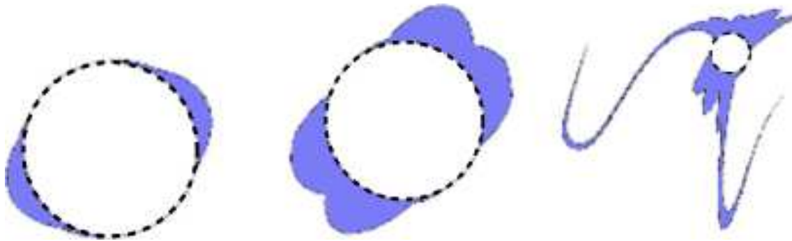
Figure 2. Initial positions of particles which have collided with a reference particle at the origin after a certain time (shaded regions). The collision region (disk of radius 2a ) is bounded by a dashed circle. At short times this region extends along the direction of the stable eigenvector of the initial flow. At intermediate times, we see the effect of this eigenvector having rotated. At long times, the set of colliding initial conditions is stretched and folded. The shaded region then covers most of the surface of the circle, including the region where the radial velocity is inward. The figure shows results of a simulated flow with small Kubo number, of the type discussed in section 4, at times t = 20\tau , t = 100\tau and t = 1000\tau .
