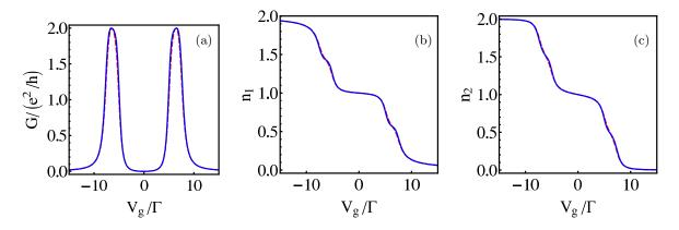
FIG. 3: (color online) Side coupled double dot with large interdot hopping:  $t_{12}/\Gamma = 4$ ,  $U/\Gamma = 8$ ,  $\Gamma_1^L = \Gamma_1^R = \Gamma/2$ , full lines: truncation order m = 4, dashed lines: truncation order m = 2, (a) conductance  $\mathcal{G}$ , (b) occupancy of directly coupled dot  $n_1$ , (c) occupancy of side coupled dot  $n_2$ .
