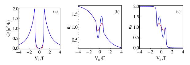
FIG. 6: (color online) Side coupled double dot with small interdot hopping  $t_{12}/\Gamma = .2$ ,  $U/\Gamma = 2$ . Other parameters and notation as in Fig. 3
