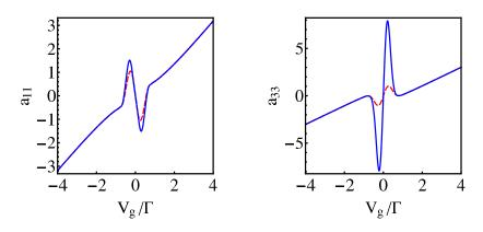
FIG. 7: (color online) Energy eigenvalues of the spin up level in directly coupled dot  $(a_{11})$  and the indirectly coupled dot  $(a_{33})$  as a function of the gate voltage for the parameter set of Fig. 6.
