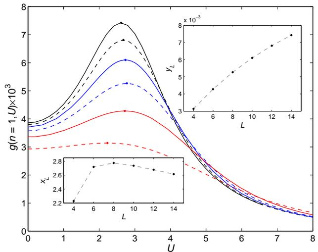
Figure 3: Scaling behavior of the intensive fidelity tensor at half filling. Dashed curves correspond, from bottom to top, to  $L = 4, 8, 12$  (antiperiodic BC's), while solid curves, again from bottom to top, to  $L = 6, 10, 14$  (periodic BC's). Note that at half filling  $g(U)$  is symmetric around  $U = 0$ . In the insets the scaling of the position ( $x_L$ ) and the height ( $y_L$ ) of the maxima is shown.
