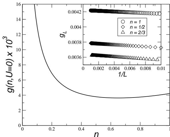
Figure 2: Fidelity metric  $g$  as a function of the total density at  $U = 0$ . The singularity at  $n \rightarrow 0$  is of the form  $n^{-1}$ . In the inset the finite size scaling of  $g_L$  for some different fillings is shown. The approach to the thermodynamic value is given by Eq. (5) with  $B = 0$ . In fact fitting the data points with Eq. (5) gives values of  $B/A$  of the order of  $10^{-4}$  and a chi-square of the same order as the one obtained with  $B = 0$ .
