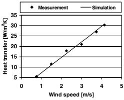
Fig. 8. Average forced convection heat transfer coefficient vs. wind speed.
