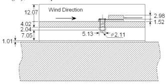
Fig. 3. Side view of the amplifier with the radiator.
