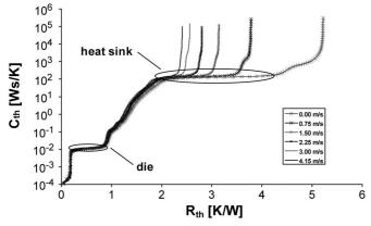
Fig. 6. Cumulative structure function.
