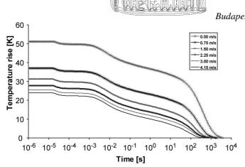
Fig. 5. Cooling curves for variable wind speeds.
