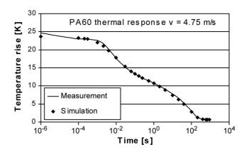
Fig. 10. Measured and simulated cooling curves - wind speed 4.15 m/s.
