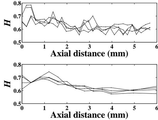
Fig. 4. Typical diagrams of Hurst exponent evolution along axial direction
