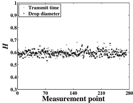
Fig. 6. Hurst exponents of transit time and drop diameter signals
