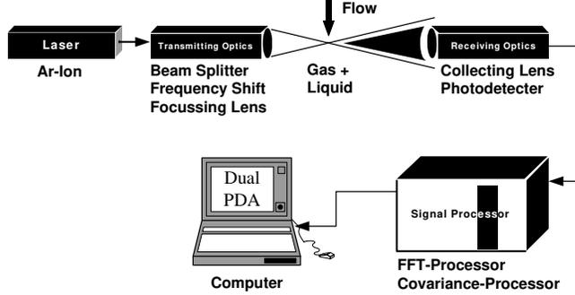
Fig. 1. Experimental set-up of the Dual PDA system
