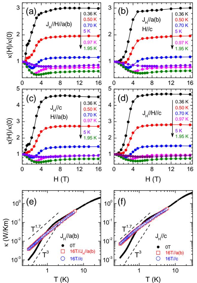
FIG. 3: (color online) (a–d) Magnetic-field dependences of the low- $T$  thermal conductivity of the  $\text{GdBaCo}_2\text{O}_{5+x}$  single crystal with  $x = 0.50$ . Directions of the heat current ( $J_H$ ) and the magnetic field ( $H$ ) are shown in each panel. (e,f) Temperature dependences of  $\kappa_{ab}$  and  $\kappa_c$  in zero and 16 T magnetic fields. The dashed lines indicate the  $T^3$  and  $T^{1.7}$  dependences.
