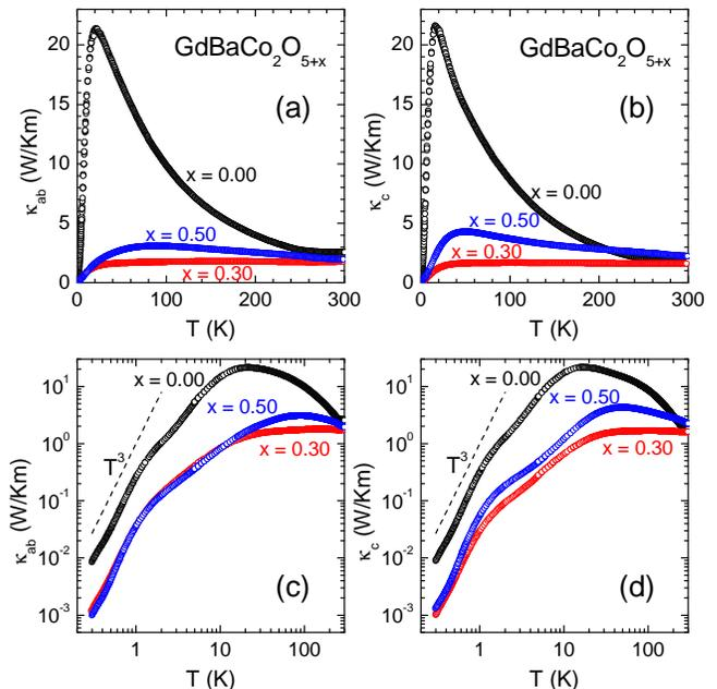
FIG. 2: (color online) Temperature dependences of the thermal conductivity along the  $ab$  plane and the  $c$  axis in zero magnetic field for  $\text{GdBaCo}_2\text{O}_{5+x}$  single crystals with various oxygen content. The data are displayed in both linear and logarithmic plots. The dashed lines indicate the  $T^3$  dependence.
