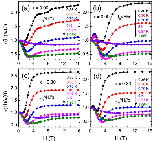
FIG. 5: (color online) Representative data for the magnetic-field dependences of the low- $T$  thermal conductivity of GdBaCo<sub>2</sub>O<sub>5+x</sub> single crystals with  $x = 0.00$  and  $0.30$ .
