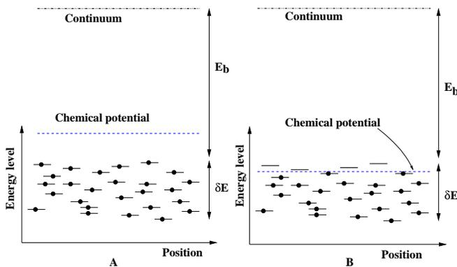
FIG. 1: The diagram of impurity energy levels. **A**: Chemical potential is outside of the impurity band. **B**: Chemical potential is inside the impurity band.  $E_b \sim 10 - 15meV$  is the binding energy, and  $\delta E$  is the width of the impurity band.
