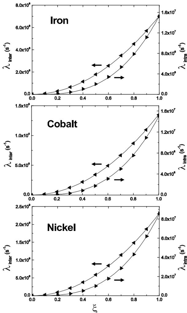
FIG. 3:  $\xi$  dependence of intraband and interband damping rates. Damping rates were calculated for a range of spin-orbit interaction strengths between off ( $\xi = 0$ ) and full strength ( $\xi = 1$ ).  $\xi^2$  fits were made to the interband damping rates (left axes and  $\blacktriangleleft$  symbols) and  $\xi^3$  fits to the intraband rates (right axes and  $\blacktriangleright$  symbols).
