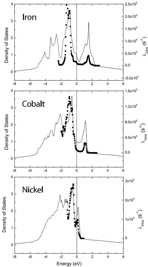
FIG. 2: Intraband damping rate versus Fermi level superimposed upon density of states. A strong correlation between the intraband damping rate versus Fermi level ( $\bullet$ ) and the density of states (solid curves) is observed. Vertical black lines indicate true Fermi energy calculated by density functional theory.
