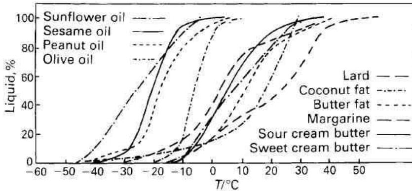
**Figure 6:** Melting curves of different natural fats.
