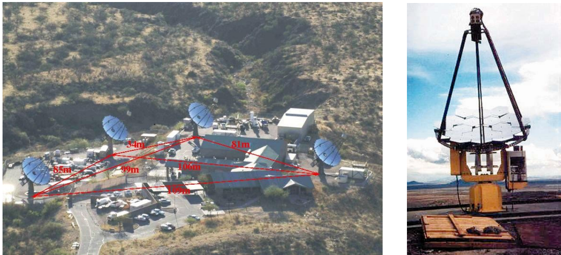
FIGURE 6. The VERITAS array, shown on the left, consists of 4 telescopes, 12m in diameter with inter-telescope baselines ranging from 34m to 109m. Before using these instruments, two 3m telescopes such as the one shown on the right are being installed in Utah for prototyping.
