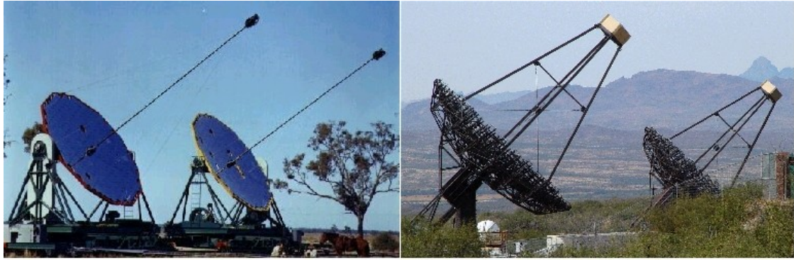
FIGURE 2. The two telescopes used in the Narrabri Interferometer are shown on the left. The two first VERITAS telescopes shown on the right could also be used as an interferometric pair of receivers.
