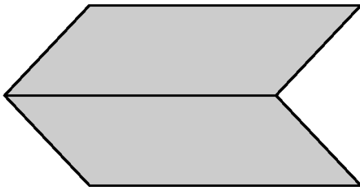
Figure 1 An ambiguous drawing: It can be interpreted as a folded paper with its edge inward or outward of the plane of the drawing.
