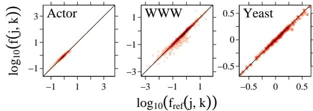
FIG. 1: (color online) Density plot of the correlation function  $f_{\text{ref}}(j, k)$  of the empirical network versus the correlation function  $f(j, k)$  of the corresponding random network as generated by the algorithm for all indices  $j$  and  $k$ . Darker red regions contain a higher density of data points, while lighter red indicates a lower density. The reference line  $y = x$  is drawn as a guide to the eye.
