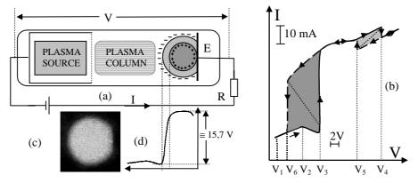
**Figure 1.** Schematic representation of the Ar plasma diode and the internal space charge configuration of the fireball (a), photograph of the fireball (b), potential drop on the double layer bordering the fireball (c), and static I(V) characteristic of the plasma diode (d).
