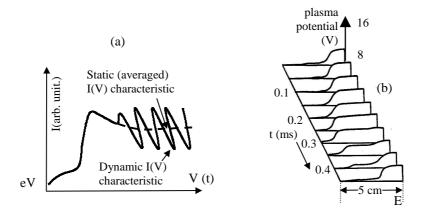
**Figure 2.** (a) Dynamic I(V) characteristic, and (b) space-time picture proving the detachment, motion and disruption of the double layer from the fireball's border.
