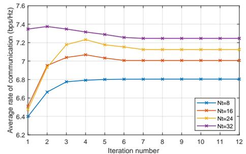
(b) The average rate of communication versus the number of iterations for  $N_t = 8, 16, 24, 32$ .
