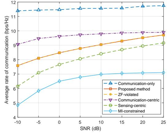
Fig. 5. The average rate of the MU-MIMO communication versus SNR.
