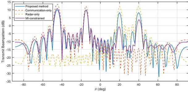
(b) The optimized transmit beampatterns with  $K = 2$ .
