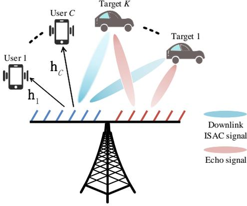
Fig. 1. Illustration of the ISAC scenario where the BS serves  $C$  downlink communication users while detecting  $K$  targets.
