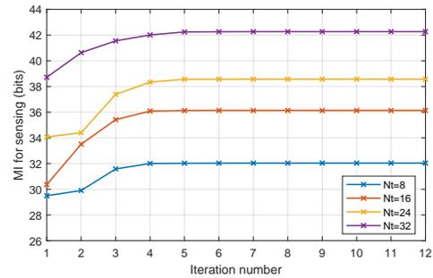
(a) The sensing MI versus the number of iterations for  $N_t = 8, 16, 24, 32$ .
