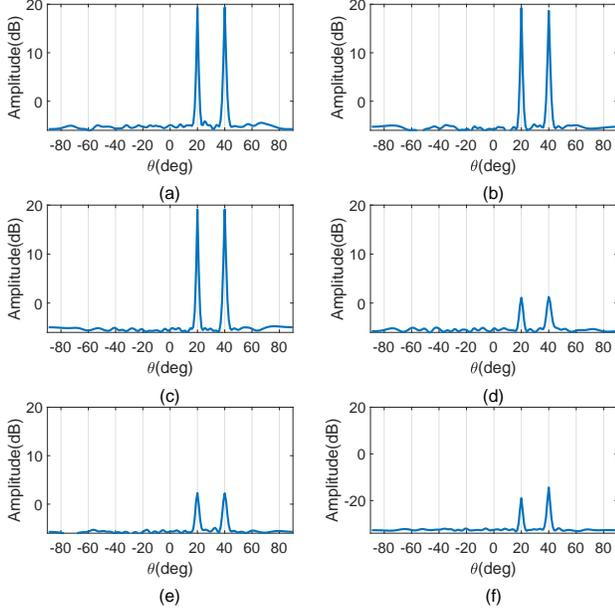
Fig. 7. Capon spatial spectrum, for  $K = 2$ . (a) Capon spatial spectrum for the Radar-only approach without radar signals. (b) Capon spatial spectrum for the proposed method. (c) Capon spatial spectrum for the proposed method without radar signals. (d) Capon spatial spectrum for the ZF-violated scheme. (e) Capon spatial spectrum for the ZF-violated scheme without radar signals. (f) Capon spatial spectrum for the MI-constrained scheme.
