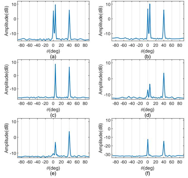
Fig. 8. Capon spatial spectrum, for  $K = 3$ . (a) Capon spatial spectrum for the Radar-only approach. (b) Capon spatial spectrum for the proposed method. (c) Capon spatial spectrum for the proposed method without radar signals. (d) Capon spatial spectrum for the ZF-violated scheme. (e) Capon spatial spectrum for the ZF-violated scheme without radar signals. (f) Capon spatial spectrum for the MI-constrained scheme.
