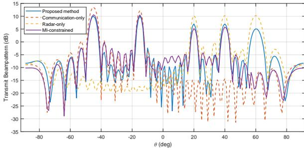
(a) The optimized transmit beampatterns with  $K = 3$ .
