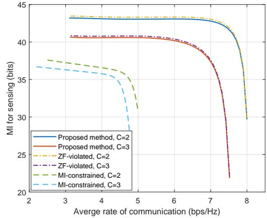
Fig. 6. The tradeoff between the sensing MI and the average rate of the MU-MIMO communication.
