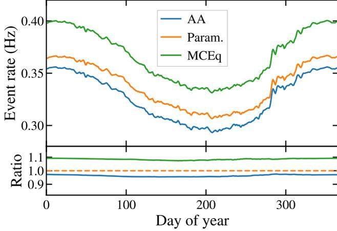
Figure 2: Daily event rate for the detector of Table 1 calculated following the three different methods from Sections 2.1, 2.2 and 2.3. (The sharp increase in the expected rate around October is a feature of the South Pole atmosphere, see for example Ref. [23].)
