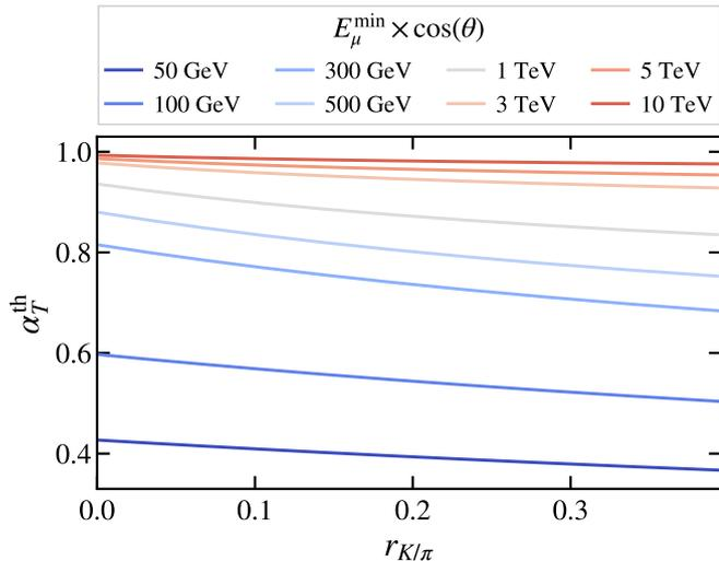
Figure 9: Theoretical expectations of the relation between  $\alpha_T$  and the kaon-to-pion ratio  $r_{K/\pi}$  calculated with the analytical approximation of the production spectrum given by Eq. (18). Spectrum weighted moments were assumed to be independent of energy.
