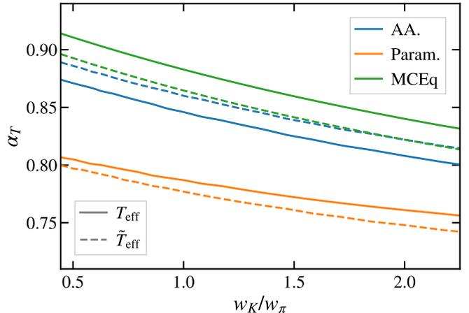
Figure 10: Relation between  $\alpha_T$  and the ratio of  $w_K$  and  $w_{\pi}$ , modifying the production of charged pions and kaons. The values are calculated for the detector of Table 1, using the analytic approximation of Section 2.1, the parameterization of Section 2.3, and the MCEq calculation of Section 2.2. Both definitions of effective temperature given in Section 3 are included.
