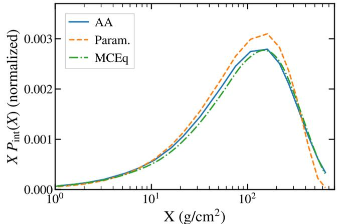
Figure 1: Integral muon production profiles obtained for  $E_\mu > 500$  GeV and  $\cos(\theta) = 0.95$  using three different methods: the analytic approximation (AA, Section 2.1), the numerical solver (MCEq, Section 2.2), and the parameterized air-shower production profiles integrated over the primary spectrum (Param., Section 2.3).
