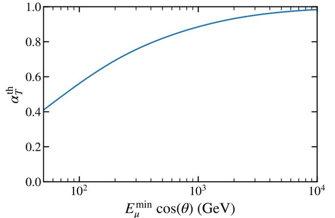
Figure 7: Theoretical prediction of the temperature correlation coefficient as a function of muon threshold energy and zenith angle, calculated using the analytic approximation of Section 2.1 assuming an isothermal atmosphere with  $T = 220$  K.
