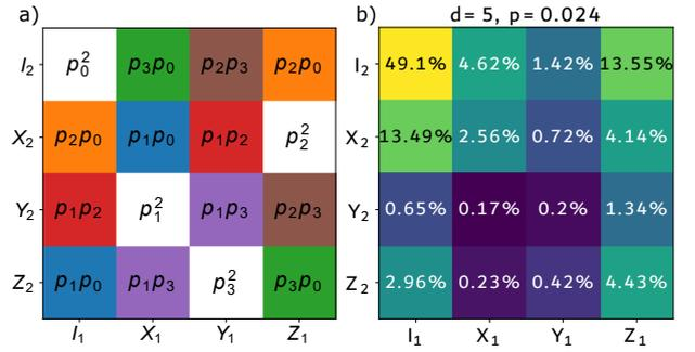
Figure 9: The structure of the two-qubit logical error channel of the lattice-surgery-based CNOT for independent noise. a) Theoretical expectation for the two-qubit logical Pauli error probabilities based on the connection parameters  $p_1, p_2, p_3$ ; non-white colors indicate symmetry partners. b) A numerically obtained two-qubit Pauli error channel that shows the expected symmetry pattern; colors indicate error rate as also written in the boxes.
