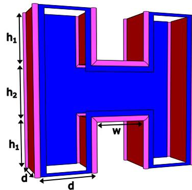
Figure 4: The spacetime diagram of the lattice-surgery-based  $\bar{Z}\bar{Z}$  measurement. Parameters are the linear size  $d$  (in data qubits) of each patch, and the length  $w$  of the "bridge" between them; and the number of measurement rounds  $h_1$  before/after, and  $h_2$  during the phase where the patches are merged.
