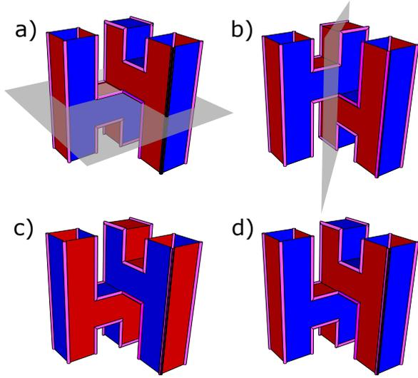
Figure 8: Symmetry of the spacetime diagram of the CNOT. For equal  $X$  and  $Z$  error rates, the syndrome graph has a symmetry transformation which consists of the following steps: 1) time reversal, 2) mirror reflection, 3) swapping the  $X$  and  $Z$  labels (colors).
