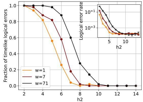
Figure 6: The fraction of timelike logical errors as a function of the number of measurement rounds during the merged phase ( $h_2$ ), for different bridge lengths  $w$ . Here,  $d = 7$ , and  $p = q = 0.006$ . The is shifted from  $h_2=7$  to smaller values for  $w = 1$ , higher values for large  $w$ , due to the higher multiplicity of timelike errors.
