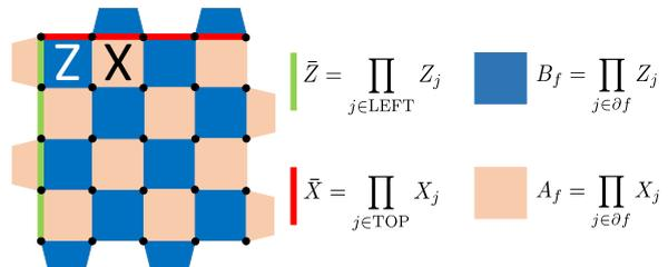
Figure 2: The layout of a distance 5 surface code patch.  $Z$ - ( $X$ -) stabilizers are products of  $Z$  ( $X$ ) operators acting on the qubits at the corners of dark (light) faces. A logical  $Z$  ( $X$ ) operator is a string of single qubit  $Z$  ( $X$ ) operators, connecting bottom (left) and top (right) boundaries depicted as a green (red) line.
