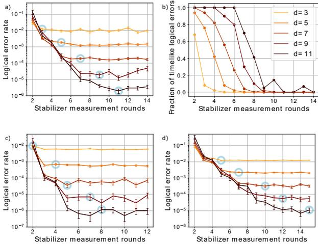
Figure 5: Errors of the  $\bar{Z}\bar{Z}$  measurement as a function of  $h_2$ , the measurement rounds in the merged phase, with  $d = 7$ ,  $h_1 = h_3 = 1$ ,  $w = 1$ , and data qubit error rate  $p = 0.6\%$ . We find that Eq.(6) (encircled values) is a decent, but not optimal choice, for readout error (a)  $q = p$ , (c)  $q = p/6$ , and (d)  $q = 3p$ . (b): The fraction of timelike logical errors for different  $h_2$  values for  $q = p$ .
