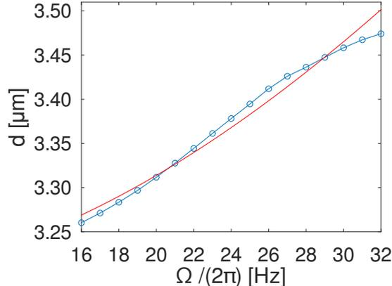
FIG. 3. Mean value of the inter-droplet distance  $d$  (blue circles) as a function of the rotation frequency  $\Omega$ . The data have been obtained by identifying the density maxima from the calculated supersolid configurations. The solid red line correspond to the distance for a non-rotating configuration with an effective trap frequency  $\tilde{\omega}_r = \sqrt{\omega_r^2 - \Omega^2}$ .
