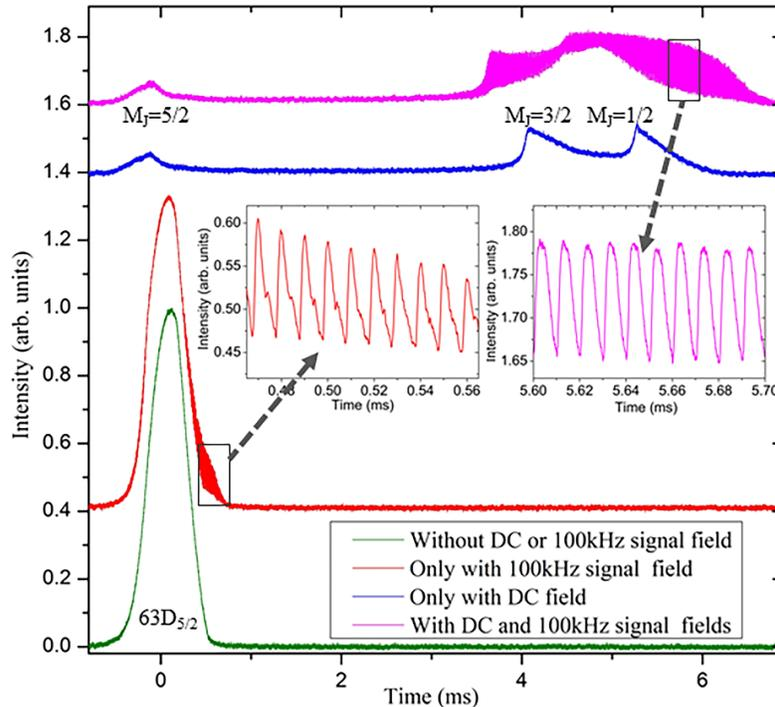
Fig. 2. EIT spectra for the Rydberg state  $63D_{5/2}$  with or without the DC and 100kHz signal field. The left and right insets magnificently display the modulations of Rydberg EIT spectra in respond to 100kHz signal field without and with the DC and field, respectively.
