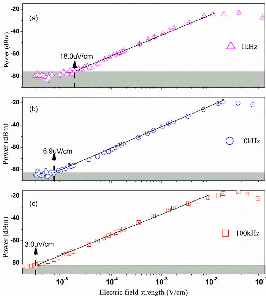
Figure 3. Strength measurement for the 1kHz (a), 10kHz (b) and 100kHz (c) signal fields using Rydberg-atom sensor. The data are taken by the spectrum analysis of the oscilloscope with an integration time of 100ms. Each data point is the average of six independent measurements, and the error bar is the standard error. The grey area represents the background noise.
