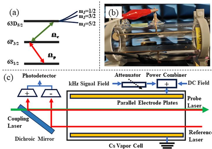
Fig. 1. (a) Relevant energy levels in cesium Rydberg EIT. (b) Photograph of Cs vapor cell with built-in parallel electrodes used in our experiments. (c) Schematic diagram of the experimental setup, including a vapor cell inside with parallel electrode plates, 852nm probe laser, 852nm reference laser, 509nm coupling laser, dichroic mirror, balanced photodetector, power combiner, DC field and kHz signal Field.
