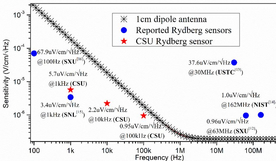
Fig. 4. Sensitivity as a function of the signal field frequency for the theoretical calculation of 1-cm dipole antenna, as well as for the reported Rydberg-atom sensors (blue circle) and our Rydberg-atom sensor (red star). Herein, CSU, SXU, USTC, SNL, NIST are, respectively, short for, Technology and Engineering Center for Space Utilization, Shanxi University, University of Science and Technology of China, Sandia National Laboratories, National Institute of Standards and Technology.
