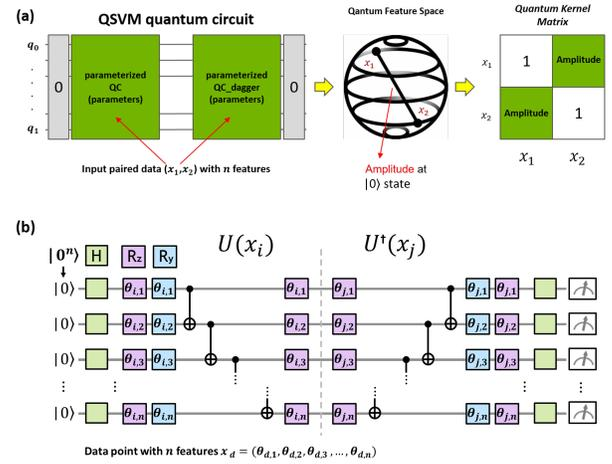
Figure 5. (a) The QSVM pipeline showcasing the quantum circuit transformation of input data into feature space quantum states. (b) A schematic of the QSVM circuit.
