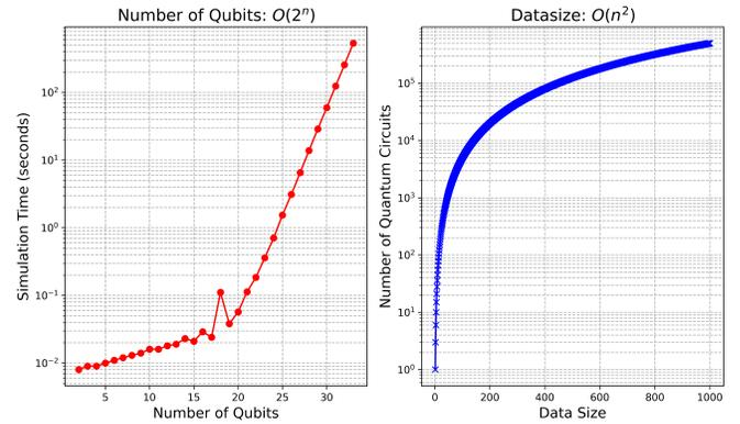
Figure 6. Computational complexity of QSVM simulation. The left graph demonstrates that simulation time scales exponentially with the number of qubits, as  $O(2^n)$ , while the right graph shows that the number of quantum circuits required scales quadratically with data size, as  $O(n^2)$ .
