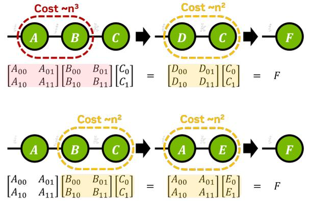
Figure 3. Consider two contraction paths: The upper path results in a higher computational cost
