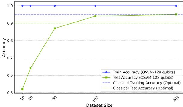
Figure 11. The relationship between dataset size and accuracy for a 128-qubit QSVM algorithm, compared to the optimal classical model.
