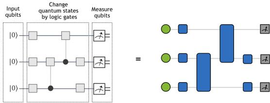
Figure 2. Quantum Circuit Formulation of cuTensorNet
