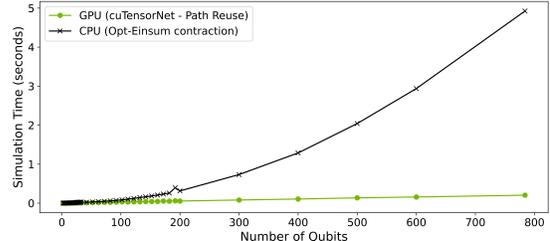
Figure 12. Benchmark QSVM circuit simulation time using a single CPU and a single GPU.
