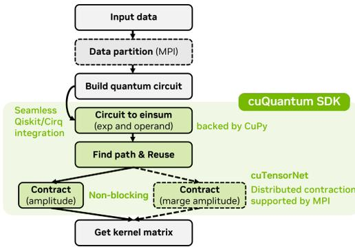
Figure 8. Workflow optimization for QSVM simulation through architectural enhancements, integrating Qiskit/Cirq with cuQuantum SDK. This transition from circuit building to tensor network conversion and kernel matrix computation reduces computational time complexity, leveraging GPU acceleration and multi-GPU strategies.
