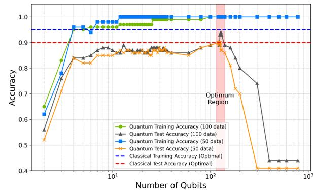
Figure 10. Train and test accuracy of quantum and classical models as a function of the number of qubits. The plot compares quantum model performance with varying training set sizes (50 and 100 data points) against the optimal classical model.
