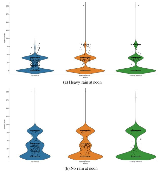
Fig. 5. Speed distribution at a curved unsignalized intersection: (a) Heavy rain at noon. (b) No rain at noon.
