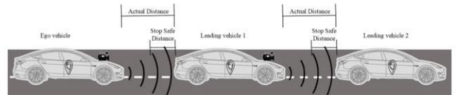
Fig. 1. Adaptive Cruise Control (ACC) model.
