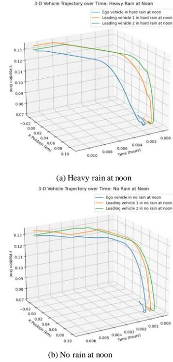
Fig. 4. 3-D vehicle trajectory over time at a curved unsignalized intersection: (a) Heavy rain at noon. (b) No rain at noon.
